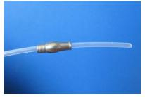
Melt the back end of the liner tube next to an open flame.... Do not stick the liner tube directly in the flame, unless you enjoy the burnt plastic smell ©.
