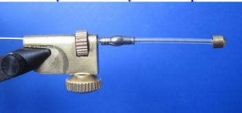
Tie on your thread securely. Make sure the Bump Tube is pushed tight against the back end of the liner tube. Make a few wraps to securely lock the Bump Tube onto the liner.
